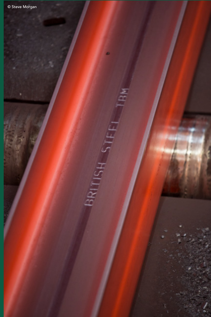
Steel Being Rolled at 1400°C, Teesside – British Steel
